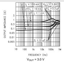
Figure 5-39. Output Impedance versus Frequency (Legacy Chip)
