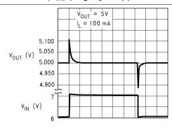
$20~\mu s/div$   $\rightarrow$   $V_{OUT} = 5~V,~I_L = 100~mA$
