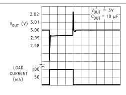
10  $\mu s/div$   $\rightarrow$   $V_{OUT} = 3.0 \text{ V, } C_{OUT} = 10 \ \mu F$
