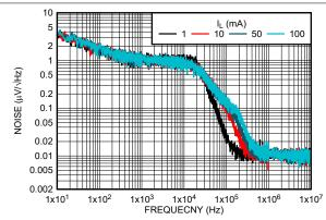
Figure 5-45. Output Noise Density versus Load Current (I<sub>L</sub>) Frequency (New Chip)
