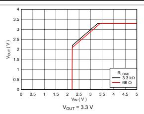
Figure 5-8. Output Voltage versus V<sub>IN</sub> (New Chip)
