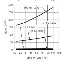
Figure 5-11. Dropout Voltage (V<sub>DO</sub>) versus Temperature (Legacy Chip)
