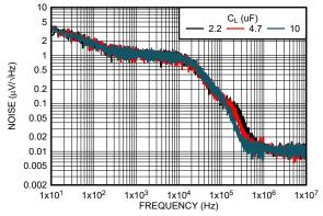
Figure 5-46. Output Noise Density versus Output Capacitor (C<sub>L</sub>) Frequency (New Chip)
