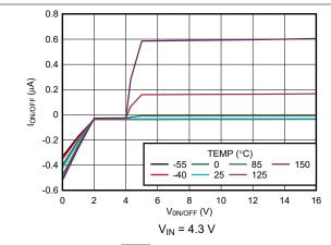
Figure 5-55. ON/  $\overline{\text{OFF}}$  Pin Current versus  $V_{\text{ON/ OFF}}$  (New Chip)
