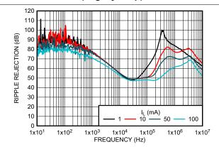
Figure 5-42. Ripple Rejection versus Load Current (I<sub>L</sub>) & Frequency (New Chip)
