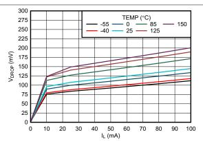
Figure 5-14. Dropout Voltage (V<sub>DO</sub>) versus Load **Current (New Chip)**
