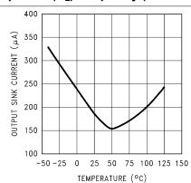
Figure 5-48. Output Reverse Leakage versus Temperature (Legacy Chip)
