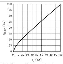
Figure 5-13. Dropout Voltage (V<sub>DO</sub>) versus Load **Current (Legacy Chip)**
