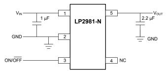
\*ON/ OFF input must be actively terminated. Tie to V<sub>IN</sub> if this function is not to be used. Minimum output capacitance is shown to insure stability over full load current range. More capacitance provides superior dynamic performance and additional stability margin (see Section 7.1.1).
