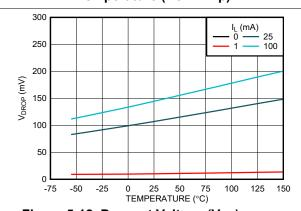
Figure 5-12. Dropout Voltage (V<sub>DO</sub>) versus Temperature (New Chip)
