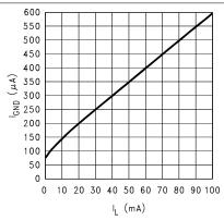
Figure 5-17. Ground Pin Current (I<sub>GND</sub>) versus Load | Figure 5-18. Ground Pin Current (I<sub>GND</sub>) versus Load **Current (Legacy Chip)**
