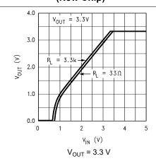
Figure 5-6. Output Voltage versus V<sub>IN</sub> (Legacy Chip)
