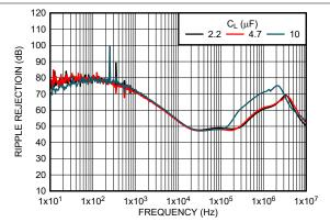
Figure 5-43. Ripple Rejection versus Output Capacitor (C<sub>L</sub>) & Frequency (New Chip)
