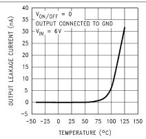
Figure 5-47. Input-to-Output Leakage versus Temperature (Legacy Chip)
