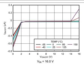
Figure 5-56. ON/ OFF Pin Current versus V<sub>ON/ OFF</sub> (New Chip)
