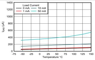
Figure 5-16. Ground Pin Current (I<sub>GND</sub>) versus **Temperature (New Chip)**
