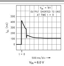
Figure 5-31. Short Circuit Current versus Time (Legacy Chip)
