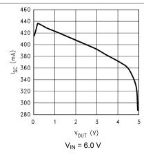
Figure 5-37. Short Circuit Current versus Output Voltage (V<sub>OUT</sub>) (Legacy Chip)
