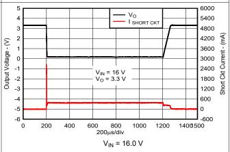
Figure 5-34. Short Circuit Current versus Time (New Chip)
