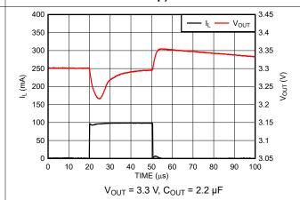
Figure 5-30. Load Transient Response (New Chip)
