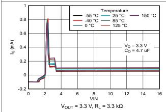
Figure 5-21. Input Current versus Input Voltage (V<sub>IN</sub>) (New Chip)
