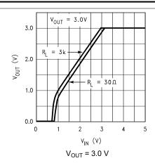
Figure 5-7. Output Voltage versus V<sub>IN</sub> (Legacy Chip)
