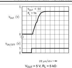
Figure 7-16. Turn-on Waveform (Legacy Chip)
