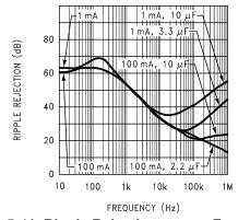
Figure 5-41. Ripple Rejection versus Frequency (Legacy Chip)
