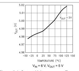
Figure 5-1. Output Voltage versus Temperature (Legacy Chip)
