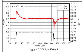
Figure 5-23. Line Transient Response (New Chip)
