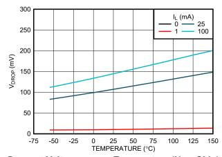
**Dropout Voltage versus Temperature (New Chip)**
