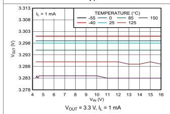
Figure 5-9. Output Voltage versus V<sub>IN</sub> and Temperature (New Chip)
