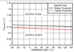
Figure 5-58. ON/ OFF Threshold versus Temperature (New Chip)
