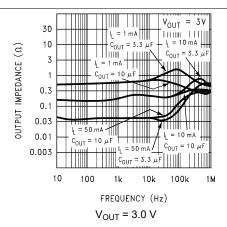
Figure 5-40. Output Impedance versus Frequency (Legacy Chip)
