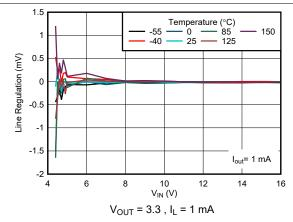
Figure 5-10. Line Regulation versus V<sub>IN</sub> & Temperature (New Chip)
