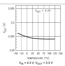
Figure 5-2. Output Voltage versus Temperature (Legacy Chip)
