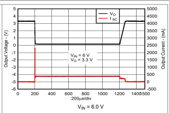
Figure 5-32. Short Circuit Current versus Time (New Chip)
