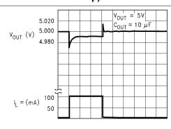
Figure 5-29. Load Transient Response (Legacy Chip)
