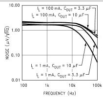
Figure 5-44. Output Noise Density versus Frequency (Legacy Chip)
