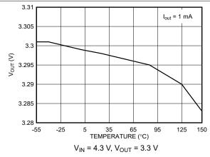
Figure 5-4. Output Voltage versus Temperature (New Chip)
