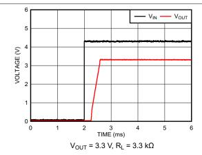
Figure 7-17. Turn-on Waveform (New Chip)
