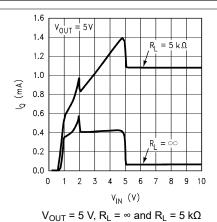
Figure 5-19. Input Current versus Input Voltage (V<sub>IN</sub>) (Legacy Chip)
