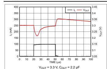
Figure 7-15. Load Transient Response (New Chip)
