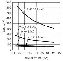
Figure 5-15. Ground Pin Current (I<sub>GND</sub>) versus **Temperature (Legacy Chip)**
