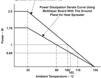
NOTE: These curves are to be used for guideline purposes only. For a particular application, a more specific thermal characterization is required.
