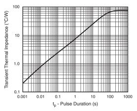
Fig. 5 - Typical Transient Thermal Impedance
