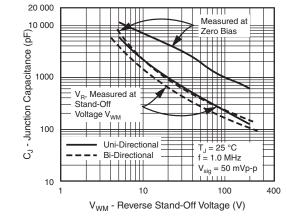
Fig. 4 - Typical Junction Capacitance Uni-Directional
