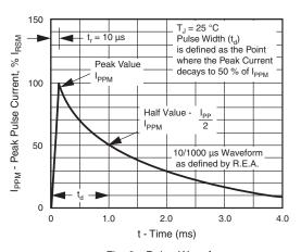
Fig. 3 - Pulse Waveform
