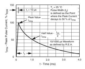
Fig. 3 - Pulse Waveform
