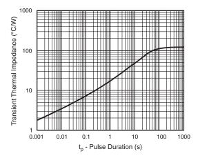
Fig. 5 - Typical Transient Thermal Impedance
