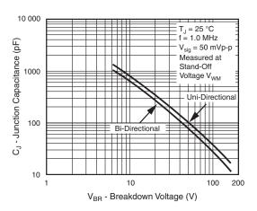
Fig. 4 - Typical Junction Capacitance
