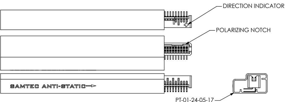
POSITION PARTS WITH POLARIZING NOTCH ORIENTED AS SHOWN
