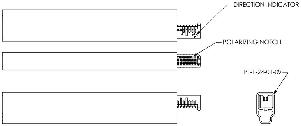
PARTS TO BE POSITIONED WITH TAILS FACING LOGO SIDE OF TUBE AND POLARIZING NOTCH ORIENTED AS SHOWN
